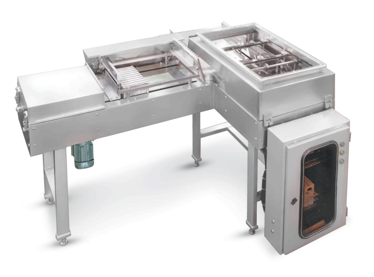
The cutting machine of this machine with stainless steel cover is designed fully automatically and with high efficiency for cutting sandwiches with desired dimensions and its control is digital.
